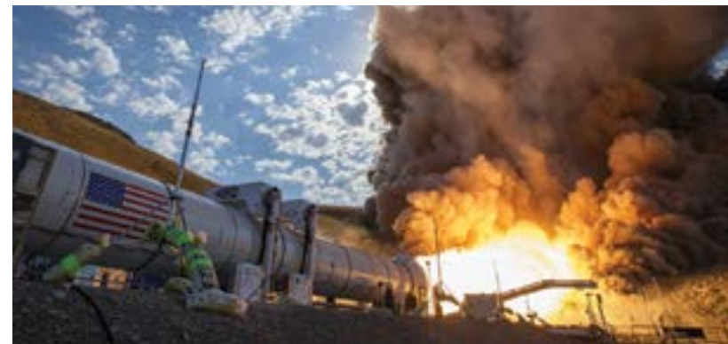
The second and final qualification motor (QM-2) test for the Space Launch System booster is seen, Tuesday, June 28, 2016, in Promontory, Utah. (NASA/Bill Ingalls)
