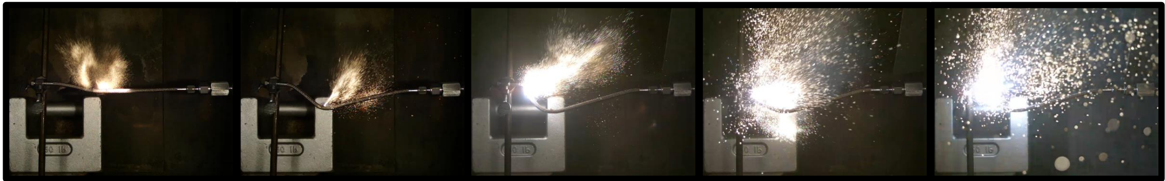
Ignition of a Teflon Hose in 1000 psi Oxygen
